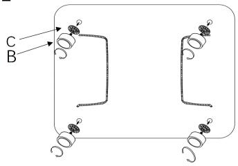
Install the legs by threading them into the pre-drilled holes as illustrated.
